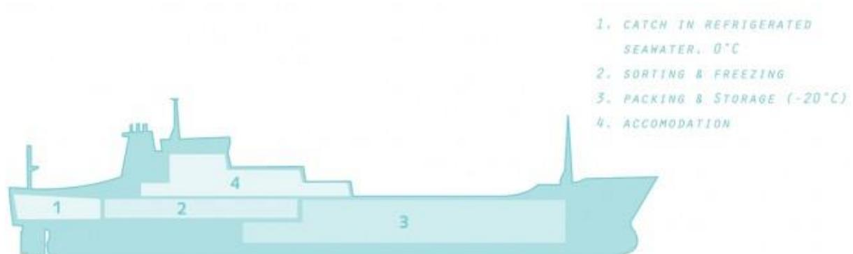
Figure 3.2. Schematic overview of a pelagic freezer trawler
