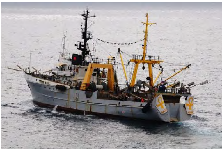
Figure 3-12. The most common type of Russian vessel in the fishery of saury.
